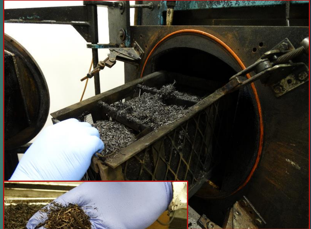
Lab scale pyrolyzer (Switchgrass 350°C)
