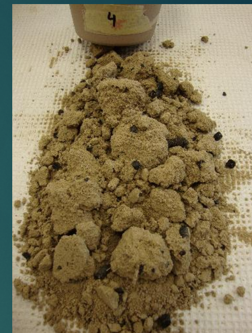
Biochar as pellets mixed into a Norfolk loamy sand
