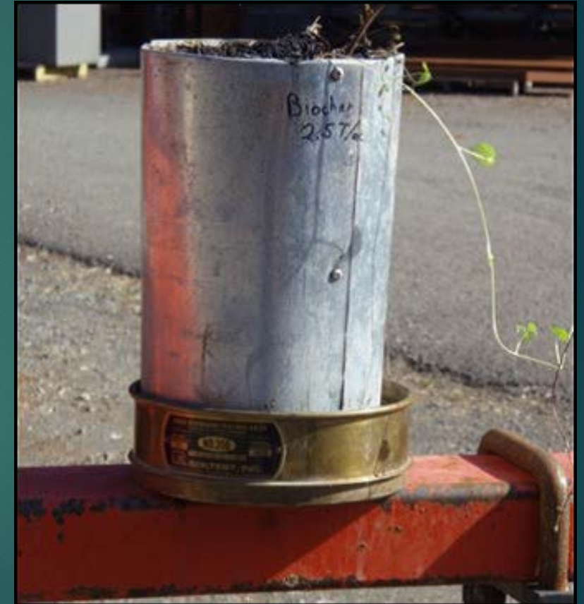
Biochar added (2.5 T/ac) to a soil test core retained more water.
