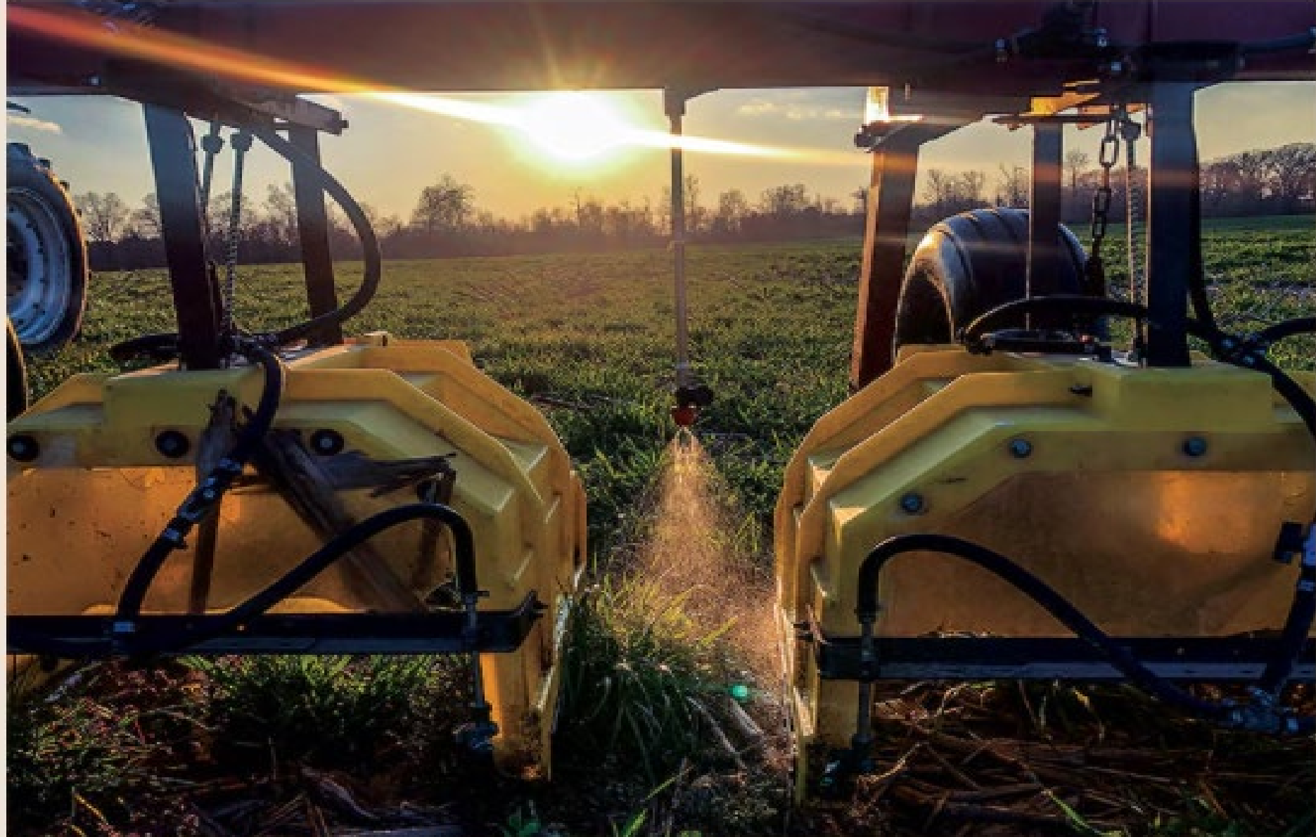
SPRAY-DOWN SKIP ZONES. Matt Griggs creates skip rows by using a hooded sprayer to terminate the cover crop in the row where the cash crop is going to be planted about two months later. Then at planting he sprays the entire field, flattens it with a roller-crimper and then plants directly into the terminated cover crop.
