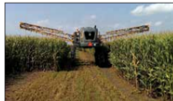
This high clearance sprayer was modified to include an air seeder. Drop tubes place the seed under the upper canopy. This works for
