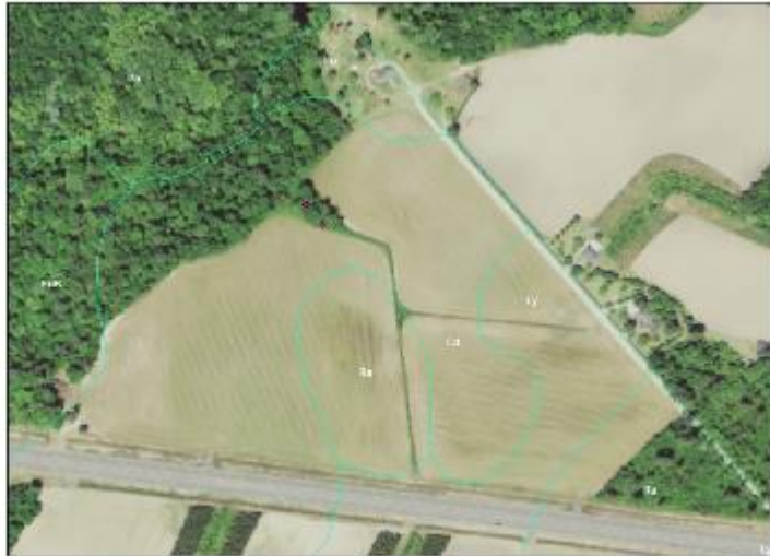
The aerial map shows the ditches that drain the land into Douglas Swamp on the Smith site. Restoration may entail blocking ditches in multiple locations, creating microtopography, thinning or narrowing planted areas, planting hardwoods and native wetland herbs, planting longleaf pine in appropriate areas; management may include removal of exotic invasive plant species, prescribed burning.
