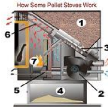
1 - Wood Pellet Hopper / 2 - Convection Fan Moves Heat 3 - Auger Feeds Pellets / 4 - Ash Pan / 5 - Automatic Igniter 6 - Heat Exchange Tubes / 7 - Burn Grate
