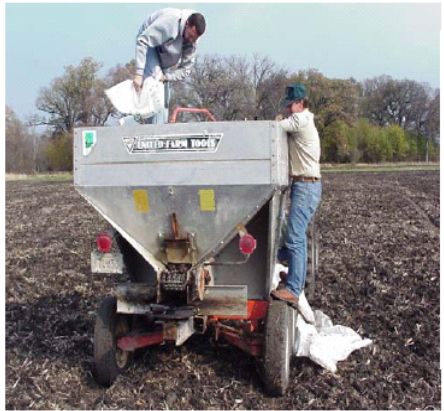
Broadcast seeding with a fertilizer buggy.
