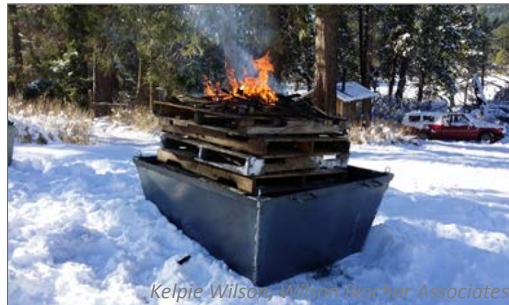
Oregon kiln, for on-site biochar production
