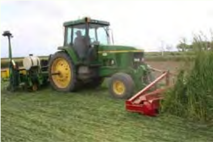
Front-mounted roller crushing fall-planted rye cover crop; planter on rear
