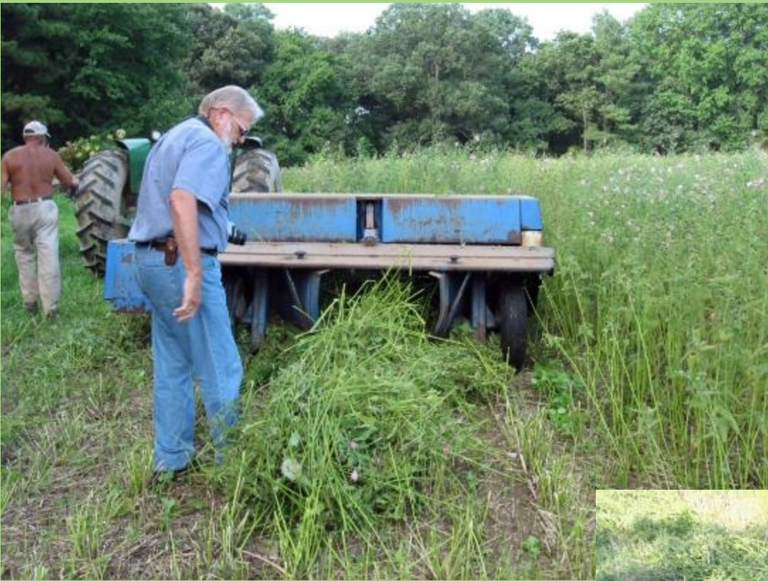
Ford hay conditioner with crimping rollers held apart
