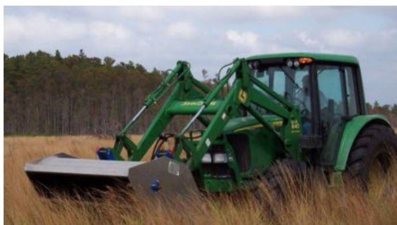
Figure 13. Proper positioning of flail-vac while collecting wiregrass seed at Three Lakes WMA. (Photo by Steve Glass)
