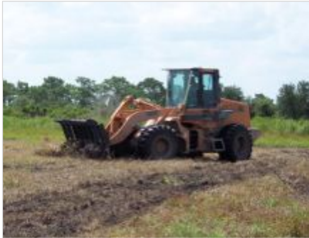
Figure 4. Root raking is part of groundcover restoration site preparations at Three Lakes WMA. (Photo by Steve Glass)
