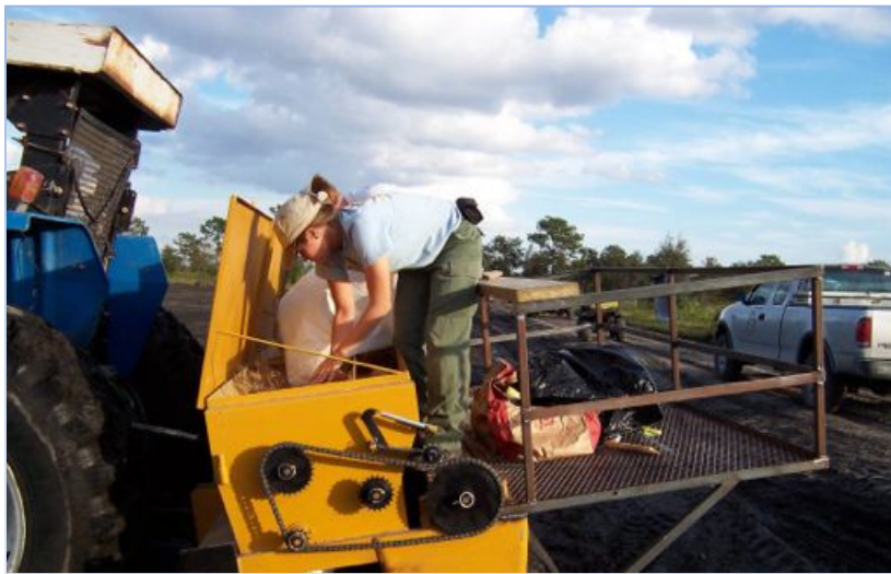
Figure 17. Custom seating and storage rack built for 8 ft Grasslander
