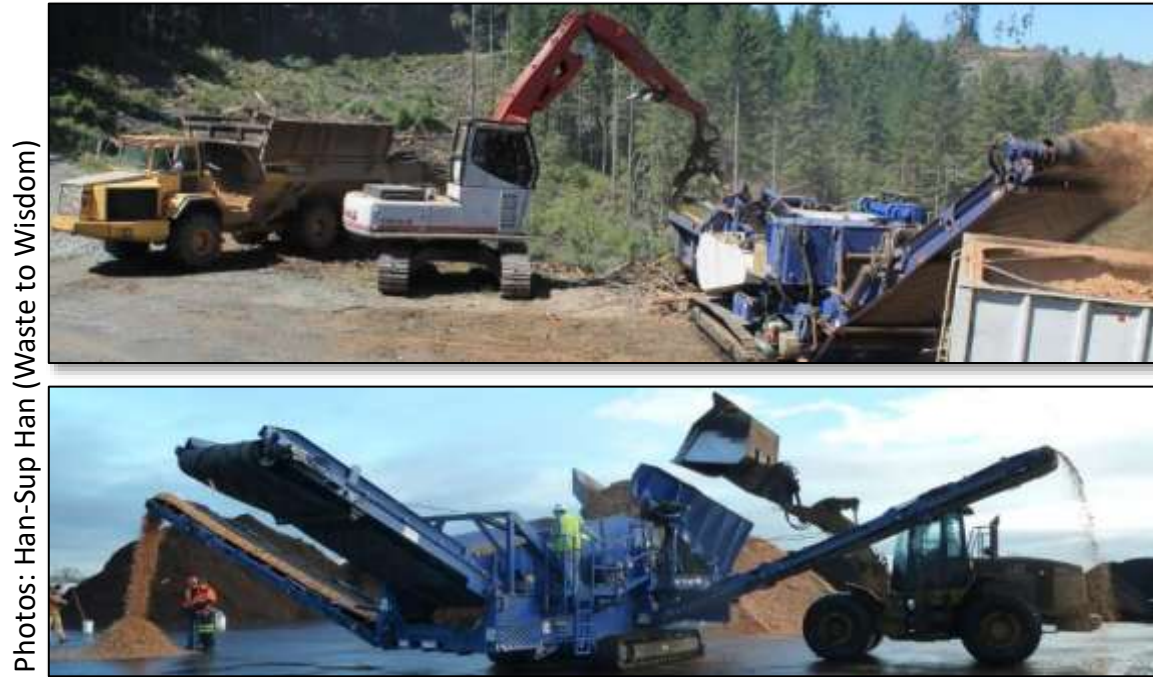
Testing alternative anvil, grate and screen configurations to increase value (W2W).
