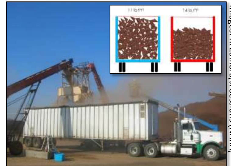
Experimental chip flinger to increase load density (NARA)
