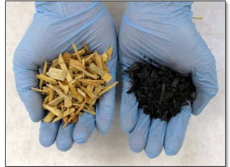
Chips and biochar produced from biomass harvested on the White River National Forest.
